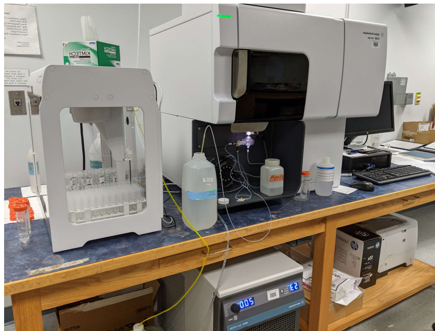
A specialized NH PHL chemistry instrument analyzes water samples for metals.
